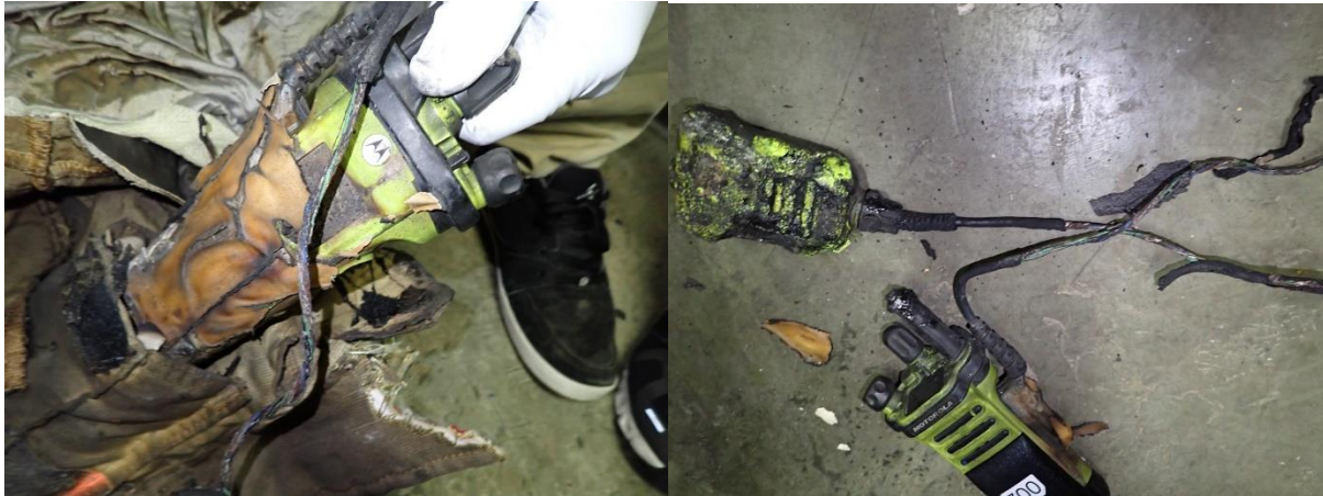
Figure 71. Tejedas radio cord burned
