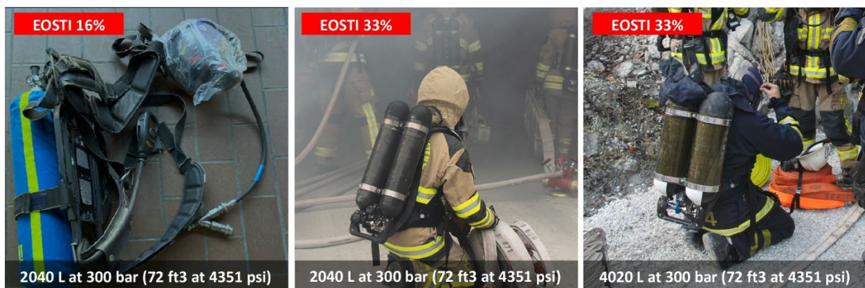
Figure 10. Self-Contained Breathing Apparatus Used in Tunnel Tests
