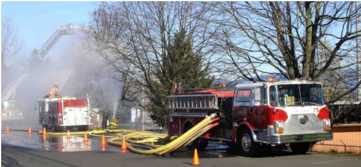
Figure 10. Gresham Fire Department Engine 79 (Training Division) Pumping for Maximum Flow
